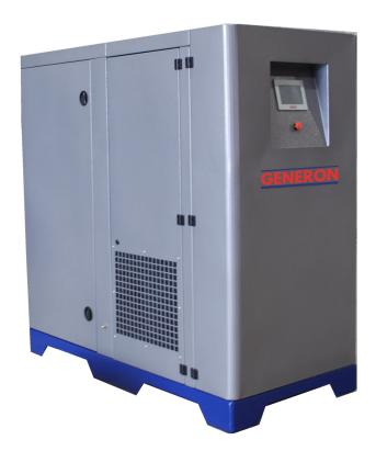
GENERON® Membrane Generators use patented High-efficiency membrane modules containing thousands of fibers. Compressed feed air is passed down the bores of the fibers at one end of the module with enriched nitrogen product gas exiting from the opposing end. Oxygen and water vapor are selectively removed from the feed air and vented as it flows to the other end of the module. These systems require low maintenance and less power to run.
